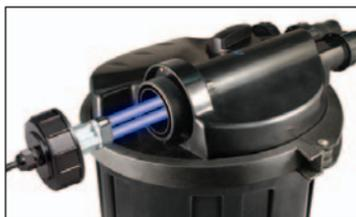
The ViaAqua® Terminator™ UVC Sterilizer is equipped with a PL UV bulb with a protected quartz sleeve that maintains the bulb temperature, thus allowing 95% of the UV radiation to clarify the water, helping to eliminate single celled free floating algae. Water resistant ballast with E-39 wire connections and over 15 feet of wire allows the ballast to be remotely mounted close to a GFCI electrical outlet.
